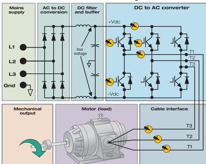
Figure 1. Basic electric schematics of variable-speed drive.
